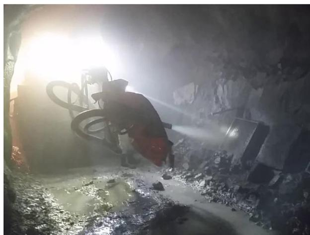
Figure 2. Sampling of the fiber reinforced sprayed concrete specimens inside a mining tunnel.
