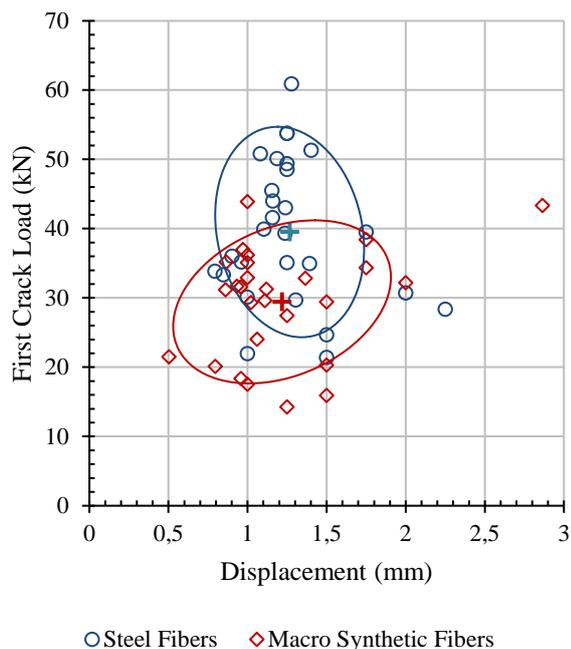
Figure 4. First crack load of FRSC specimens and confidence ellipses (95% likelihood) by fiber type obtained from EFNARC tests.
