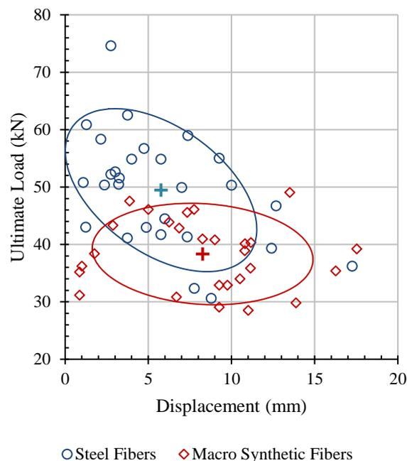
Figure 5. Ultimate load of FRSC specimens and confidence ellipses (95% likelihood) by fiber type obtained from EFNARC tests.
