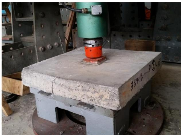
Figure 1. Energy absorption test according to EFNARC on a fiber reinforced sprayed concrete specimen.
