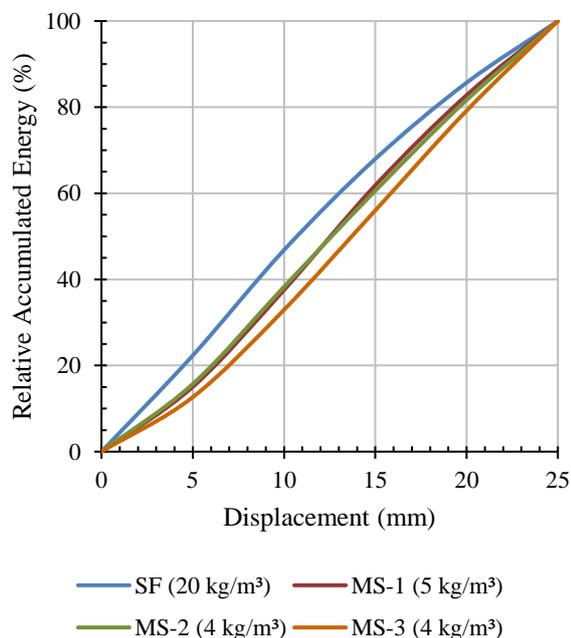
Figure 3. Relative accumulated energy ( $RAE_i$ ) obtained by sprayed concrete specimens separately reinforced with steel fibers (SF) and macro synthetic fibers (MS) with different producers and dosages on EFNARC tests.
