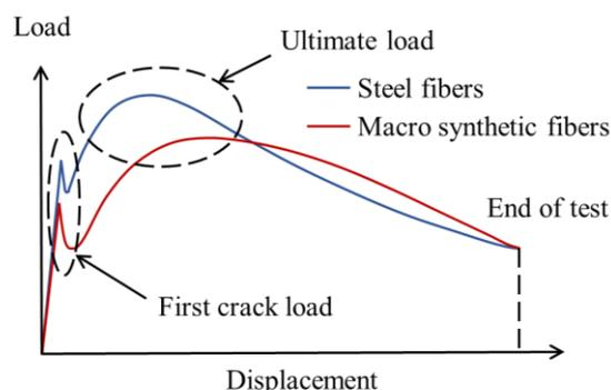
Figure 6. Typical Load-Displacement curves plotted according to values obtained from analyzed tests.
