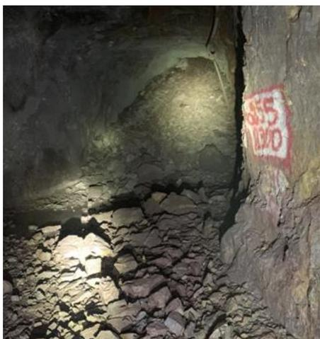
Figure 6 – Post blast results showing good fragmentation.
