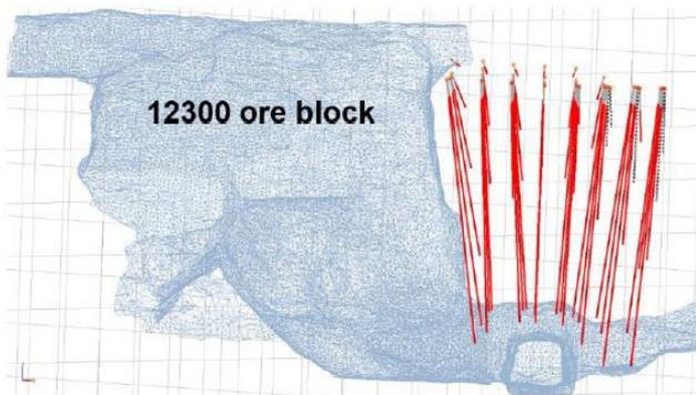
Figure 5 – BL1 12300 pillar loaded with WebGen™ 100 wireless detonators and CMS (Cavity Monitoring System) from 12300 stope
