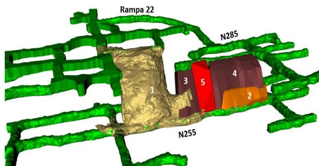
Figure 4 - layout and mine sequence from the stopes
