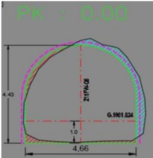
Figure 5. Topographic profile of the production level developed using equipment with computerized control (Source: Cortes Zablocki, 2018).
