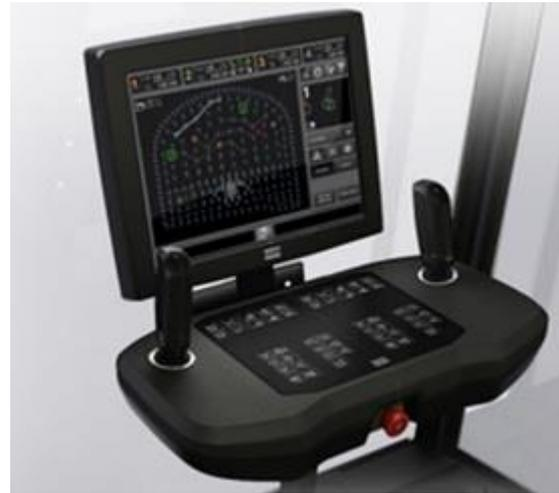
Figure 3. Rig Control System (RCS 5) (Source: Cortes Zablocki, 2018).
