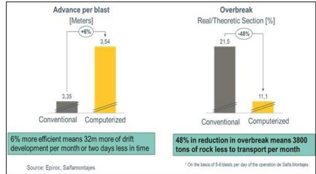
Figure 7. Comparison of conventional and computerized systems: advance-per-blast (left) and overbreak (right) (Source: Cortes Zablocki, 2018).
