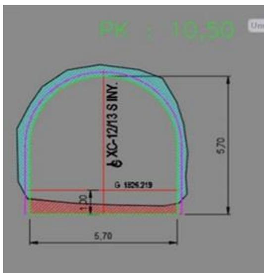
Figure 6. Topographic profile of a gallery developed with conventional equipment (Source: Cortes Zablocki, 2018).
