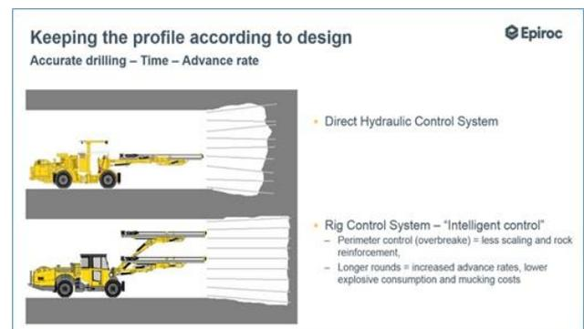
Figure 8. Benefits of computerized drilling versus manual/conventional drilling (Source: Zablocki, 2018).
